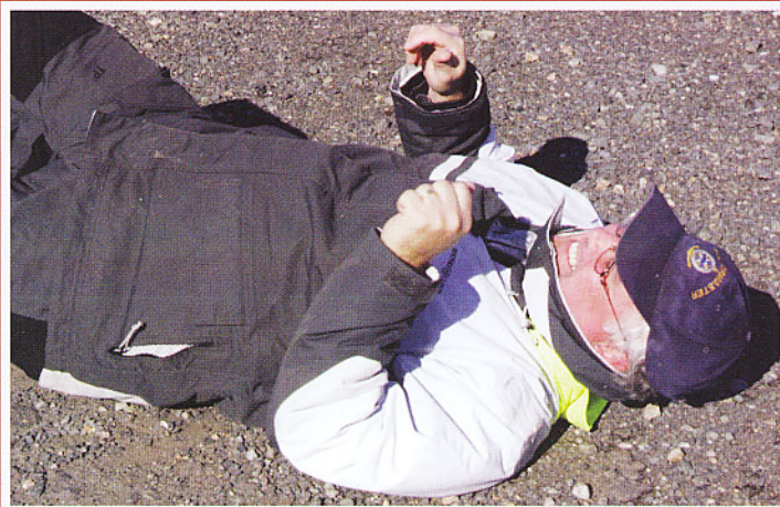
To test each garment's resistance to abrasion and wear, testers scooped across a gravel parking lot first on their bellies and then on their backs.
